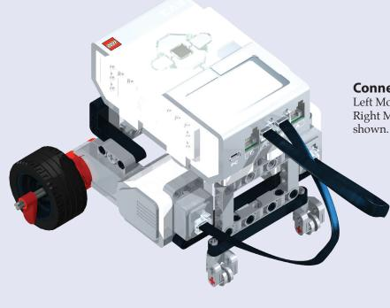
**Connecting the Cables** Left Motor connects to Outlet B and Right Motor crosses to Outlet C as shown.
