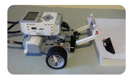
Build the Cargo Delivery Attachment from the instructions provided. Connect the Medium Motor to Port D of your EV3 brick. The Cargo Deliver arm can be raised and lowered by instructing the D motor to rotate approximately 90 degrees.
