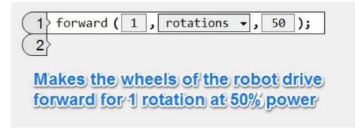
Run the program again and watch the wheels very carefully. You should notice that both wheels turned exactly 1 rotation causing the robot to drive forward a short distance. How far is this 'short distance' however? There are a few ways we can figure this out.
