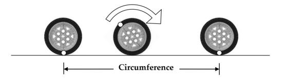
**Mathematically:** The circumference of a wheel can be calculated using the formulae:  $c=\pi \times d$
